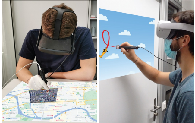
Figure 1: Flashpen is a precise pen input device that can be used in a virtual reality environment (virtual reality content superimposed in this figure to visualize system usage). The device can be used on a horizontal surface like a table (left) or a vertical surface (right).
