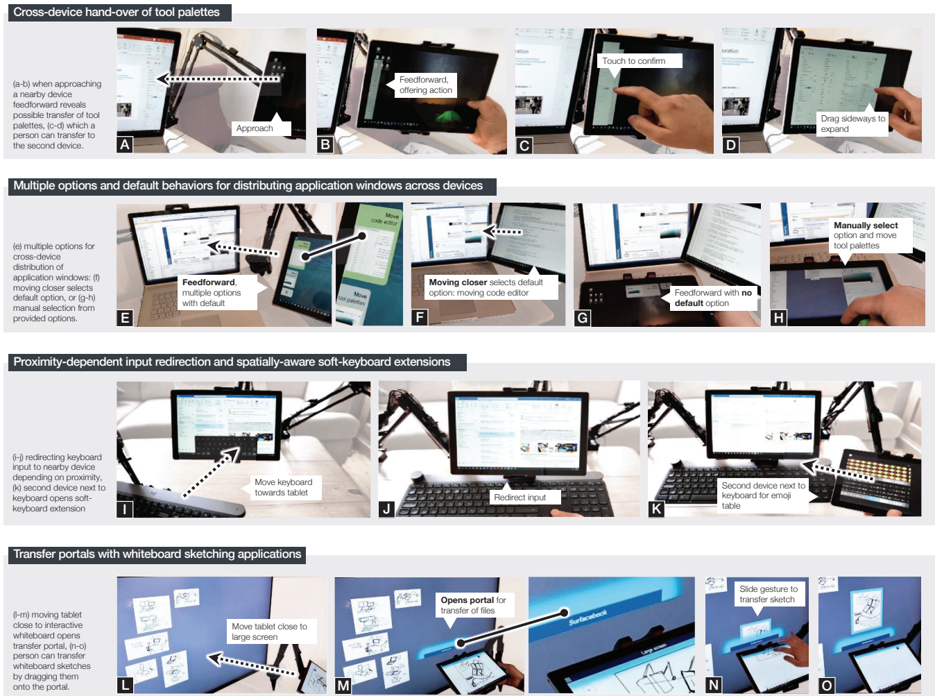
Figure 7: Productivity applications with AirConstellations: (a-d) distributing tool palettes across devices, (e-h) multiple available options for proximity-based application behavior, (i-k) proximity-dependent input redirection of physical keyboards, and spatially-aware soft-keyboard extensions, and (l-o) opening transfer portals across devices in a whiteboard application.
