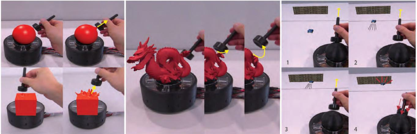
Figure 11. We present possible use cases for *Omni*. *Left* show the possibilities in 3D CAD design, in this case sculpting. *Center* shows a user is exploring and manipulating an augmented reality object. For both applications, users can feel the shape of the outer hull of the objects. *Right* shows a racing game. Once the car collides with the wall, the pen gets pushed to the base. Arrows indicate movement and are drawn on top of the photo to increase clarity.
