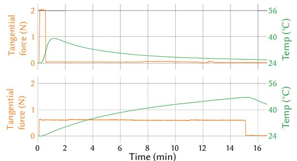
**Figure 9. Temporal evolution of the self-heating of the coils for two different types of actuation. Top: a *peak-force* of 2 N ( $I_y = 15$  A) during 25 seconds. Bottom: a *constant-force* of 600 mN ( $I_y = 5$  A) during 15 minutes.**
