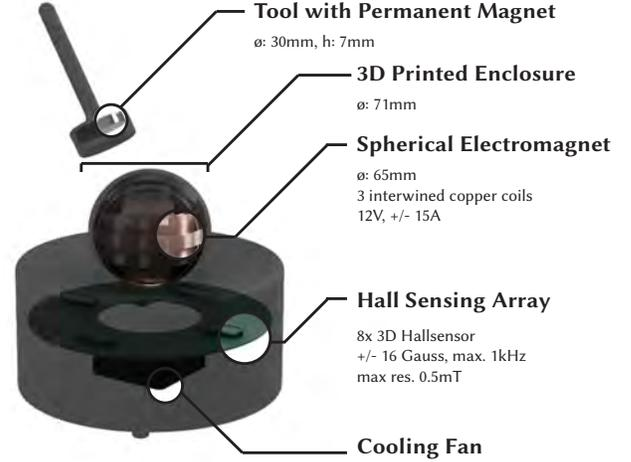
Figure 4. *Omni* hardware overview. Annotated view of the most important components of the system. All components can be acquired commercially or are easy to produce in a standard FabLab. A top-down view of the physical device can be seen in Figure 1.
