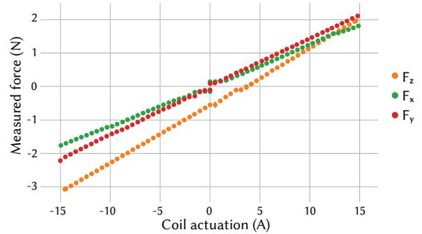
**Figure 8. Radial and tangential forces on the permanent magnet as a function of coil actuation  $I_x$ ,  $I_y$  and  $I_z$ , for the magnet located on top of the sphere (Fig 7). Force was collected with a compression-like force sensor.**
