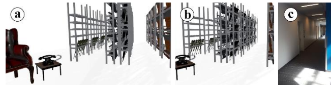
Figure 6: Real-walking enabled by eye-tracking. (a) In the loading room, the user is walking towards two lines of storage racks. (b) Mise-Unseen shifts the rack that the user appears more interested in, (c) so that the user can walk through.
