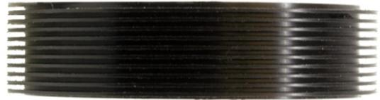
Figure 6: A helix groove machined into the acetal drum to prevent cord overlap.
