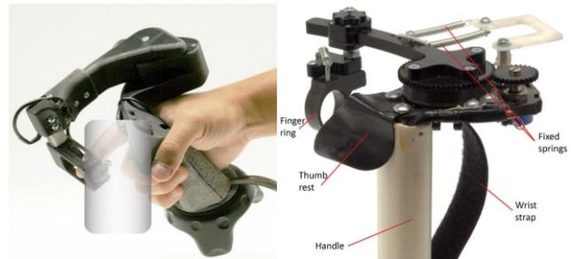
**Figure 11: Left) Claw device. Right) Fixed-Spring device.** The Spring device was built as a copycat of the other two prototypes CapstanCrunch and CLAW with the difference that the finger arm was only connected to a fixed spring.
