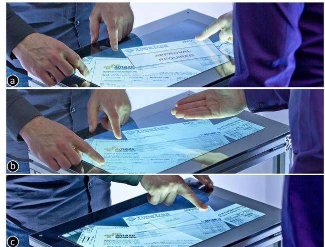
**Figure 4:** Example scenario. A bank manager (left) and clerk (right) approve invoices. (a) When the clerk encounters a bill above his approval limit, Fiberio refuses the payment. (c) The manager completes the transaction, pushing the same button.
