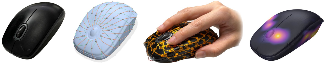
Fig. 1. We propose a computational fabrication pipeline that equips existing 3D objects with mutual-capacitance sensing for touch input. Starting from a 3D scan of a physical object (left), our method generates two layers of electrode curves that conform to the object’s surface geometry, tailoring their layout with linear optimization for sensor coverage and distribution (center). We fabricate these curves from copper foil using a vinyl cutter, attach them to the surface, and connect them to a mutual-capacitance controller for live sensing and visualization (right).
