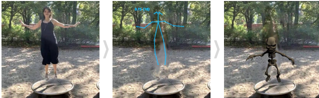
Figure 4: Examples for our 3D-pose-aware object substitution approach. 3D pose estimation is performed for vehicles (top) and humans (bottom). Vehicles poses are estimated as oriented 3D bounding boxes. Human poses are estimated as 3D joint keypoints.
