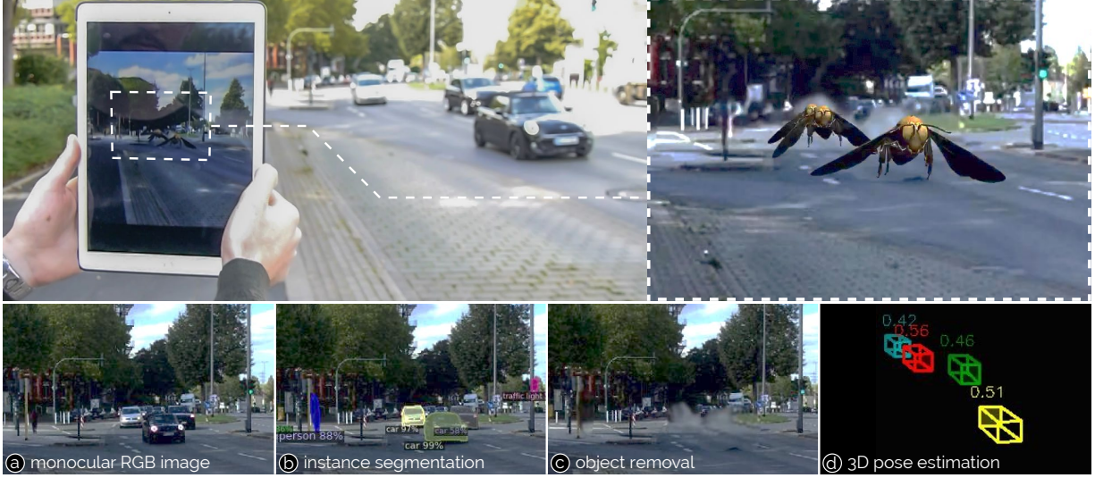
Figure 1: TransforMR is a video see-through mixed reality system for handheld devices that performs 3D pose-aware object substitution to create meaningful mixed reality scenes, enabling applications such as alternate mixed realities or real-time virtual character animation in context. (a) From just the monocular color camera of a mobile device, (b) TransforMR performs instance segmentation, (c) object removal, and (d) 3D pose estimation to substitute objects with pose awareness (top right).
