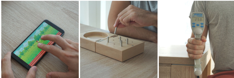
Fig. 2. Study methods: smartphone-based fatigability task on the left, nine-hole peg test centered, and handgrip dynamometer on the right.
