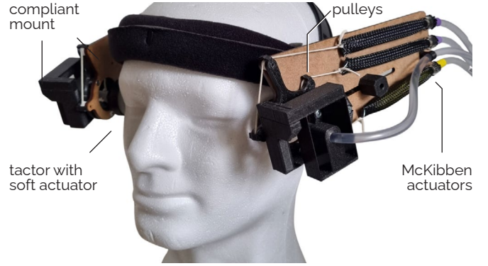
Fig. 1. MiBOT is a head-massage robot that integrates two symmetrically actuated massaging units, each mounting pneumatic artificial McKibben muscles to actuate a soft tactor on either side of the face. MiBOT dynamically adjusts the pressure applied to the wearer’s head through a sensor-driven control loop to dynamically conform to various head shapes and topological features, while performing massage motions reminiscent of human touch.
