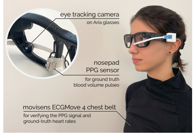
Figure 2. Apparatus used to record the egoPPG-DB dataset.
