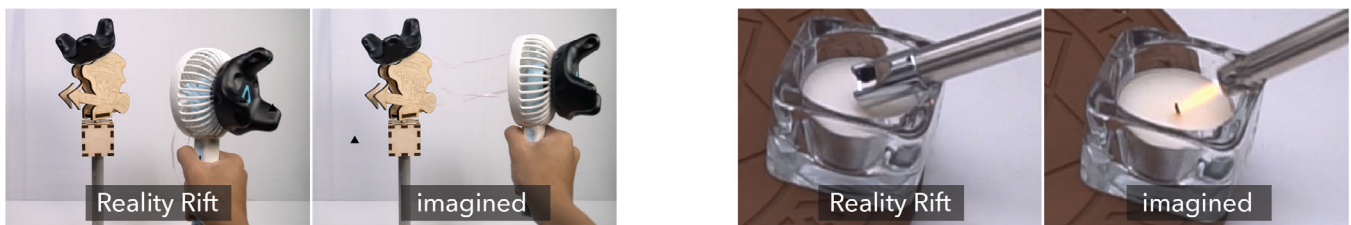
Figure 6: Left: the motorized wind vane responds to the unpowered fan resulting in the imagination of wind. Right: the candle responds to a flameless lighter resulting in the imagination of fire.
