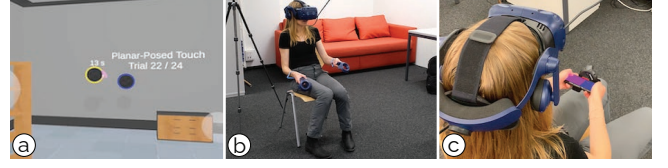
Figure 6: Apparatus for our full-range study. a) Our Unity app rendered the study environment, displayed through a VIVE Pro Eye. b) For Go-Go input, participants used the VIVE controllers. c) For all phone techniques, a VIVE tracker provided the pose of an iPhone 11 Pro, which relayed touches to Unity.
