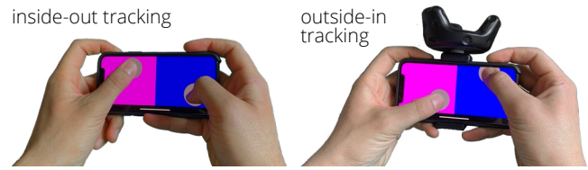
Figure 5: Users hold the HandyCast input phone like a gamepad, with each thumb operating in a single touch zone. For usage in common VR games, HandyCast can use inside-out tracking with no additional tracking hardware needed. For our two evaluations, a VIVE tracker is mounted to the phone allowing us to separately investigate interaction performance and tracking effects.
