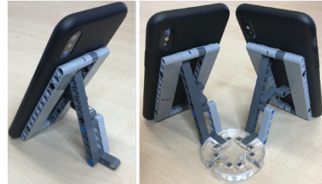
Figure 4. The smartphone case (left side) has an included stand that can be expanded and collapsed. It ensures that the smartphone can easily be placed on the table in the correct tilting angle. The connector widget (right side) allows the users to easily arrange up to four smartphones in a fixed position.
