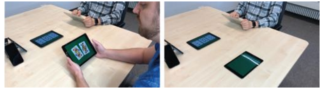
Figure 6. GazePoker prevents cheating, by continuously authenticating users in front of their cards based on their faces. When a player leaves in GazePoker, or another peeks in, those cards are hidden.
