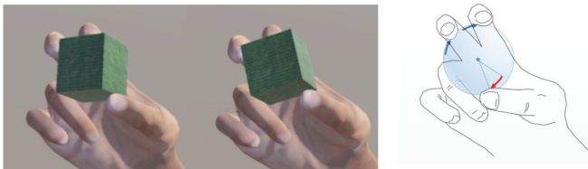
Figure 12: TORC allows precise manipulation of a held objects rotation by sensing finger motion (left). Rotation is around the center of rotation between the fingers and it is controlled by the thumb motion. The index and middle fingers rotate in the opposite direction (middle & right).
