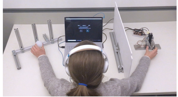
Figure 5: Experiment setup. The participant compared two rendered sensations A and B from our device (right hand) to the sensation of an analog object, a \varnothing 5.08 cm silicone ball made of Eco-flex 00-30 (durometer 27.4 (Shore hardness, scale: OO)) (left hand).
