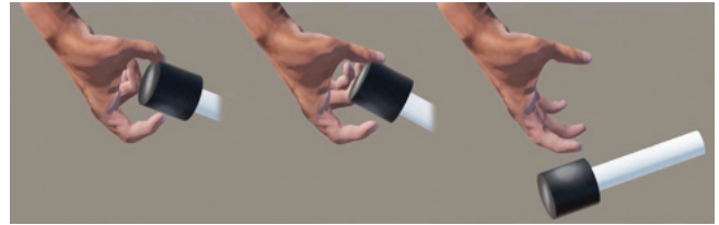
Figure 9: Fingers are holding the object, with joint position estimated by inverse kinematics (left). Applying a little pressure outward by opening the index & middle fingers releases the grabbed object (middle & right).
