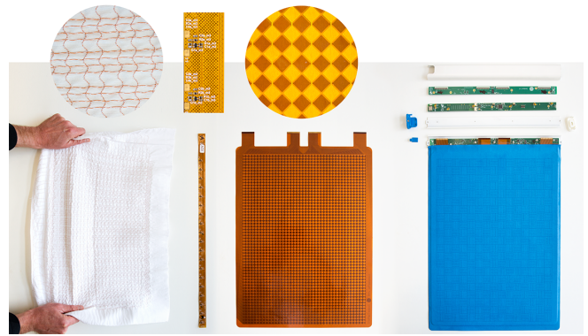
Figure 2. Zanzibar Mat components, from left to right: Stretchable NFC antenna array, flexible antenna interconnect, flexible capacitive electrode matrix, rigid PCBs housed in the baton enclosure.
