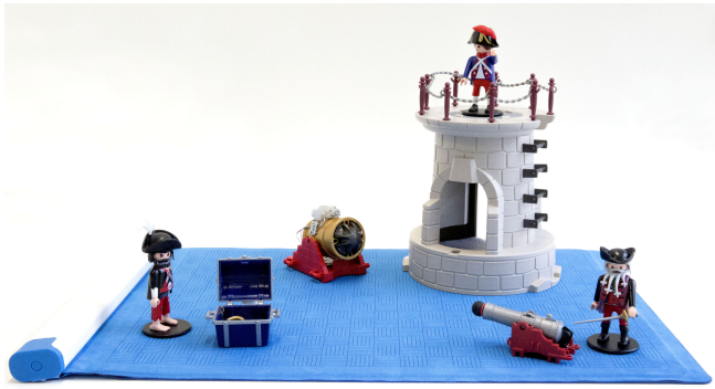
Figure 5. The Pirate Toybox screenless playset uses audio to complement physical play, which extends to the top of the tower. I/O Tags actuate and sense interaction with the chest and cannons.
