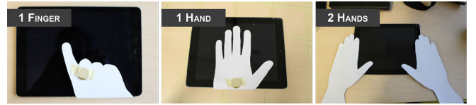
Figure 6. PolarTrack’s tracking quality was evaluated with 1-finger, 1-hand, and 2-hands occlusion.
