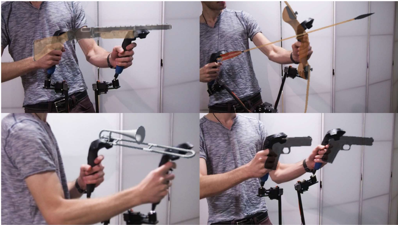
Figure 7. Objects explored in the user evaluation. Left to right, top to bottom: RIFLE, BOW, TROMBONE, PISTOLS. Overlay added in post-production for visualization.
