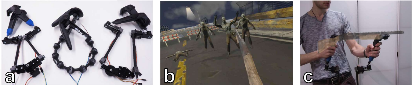
Figure 1. (a) Three prototype Haptic Links attached to commercial HTC VIVE controllers. From left to right: Layer-Hinge , Chain , Ratchet-Hinge . (b-c) A survival game in which a Haptic Link rigidly locks handheld controllers in the shape of a two-handed gun. Overlay added in post-production for visualization.
