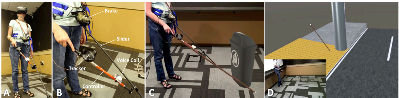
Figure 1. (A) A blind user wearing the gear for our VR evaluation, including a VR headset and Canetroller , our haptic VR controller. (B) The mechanical elements of Canetroller . (C) Overlays of the virtual scene atop the real scene show how the virtual cane extends past the tip of the Canetroller device and can interact with the virtual trash bin. (D) The use of Canetroller to navigate a virtual street crossing: the inset shows the physical environment, while the rendered image shows the corresponding virtual scene.
