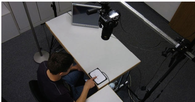
Figure 9: Participants acquired a crosshair target located on a touchpad and committed input using the footswitch.
