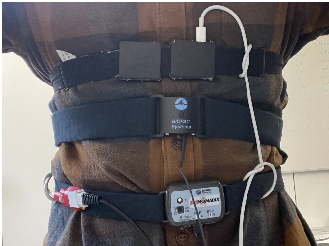
Fig. 4. The device setup on the participant’s thorax for the study included the custom UWB device which was strapped over the sternum, followed by the reference respiratory belt over the abdomen, and the transmitter of the respiratory belt.
