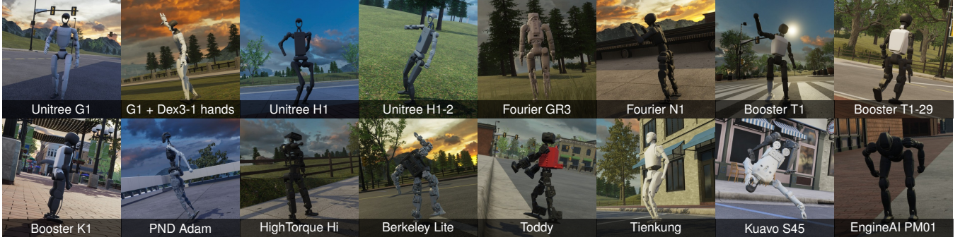
Fig. 3: The training corpus. Human motion capture retargeted onto sixteen humanoids spanning 3.0\times in height (0.60–1.78 m) and 19–43 degrees of freedom, rendered in Unreal Engine under randomized scene, illumination and viewpoint. One sample is shown per robot, paired with the configuration used to render it.
